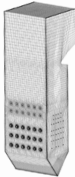
Computational mesh of the boiler
