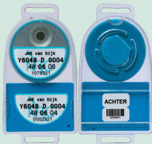
Figure 1: The neutron dosimeter consisting of the combination of a TL dosimeter (top) and a PADC dosimeter.
