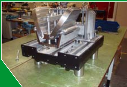
The specially designed 'butterfly' shield for the reactor core.
