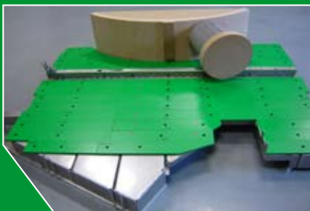
The mockup of the Densimet shielding
