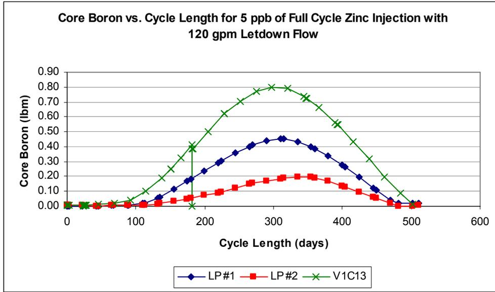
Fig 8. Boron Deposition vs. Burnup
