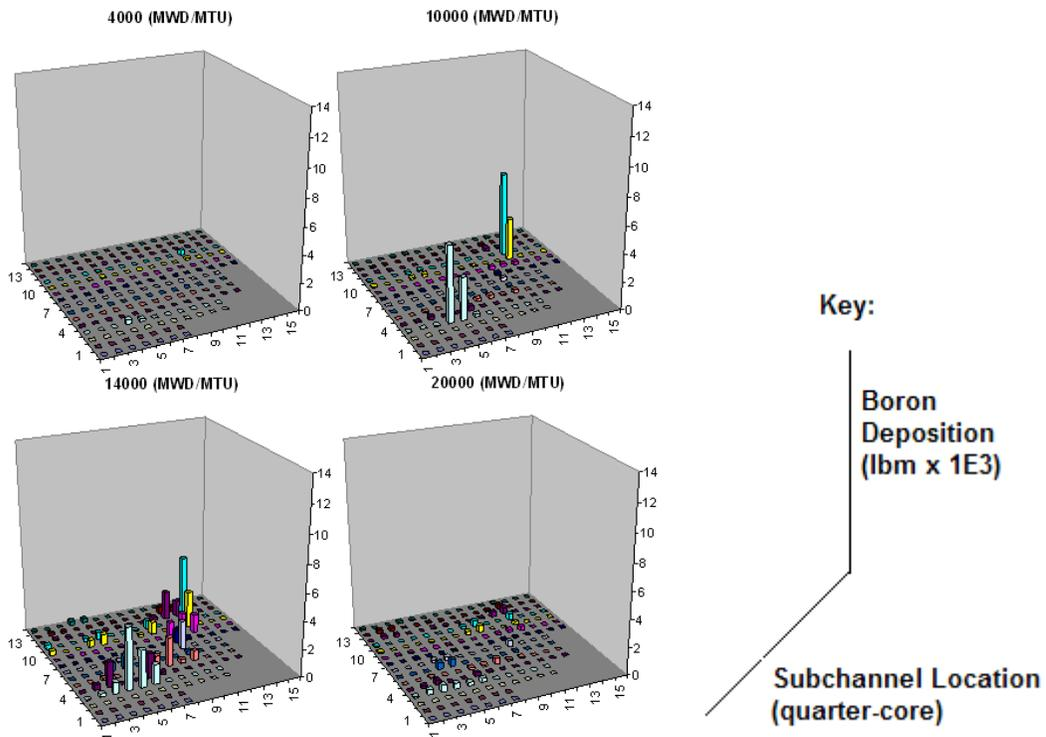
Fig 7. Boron Deposition for LP #2
