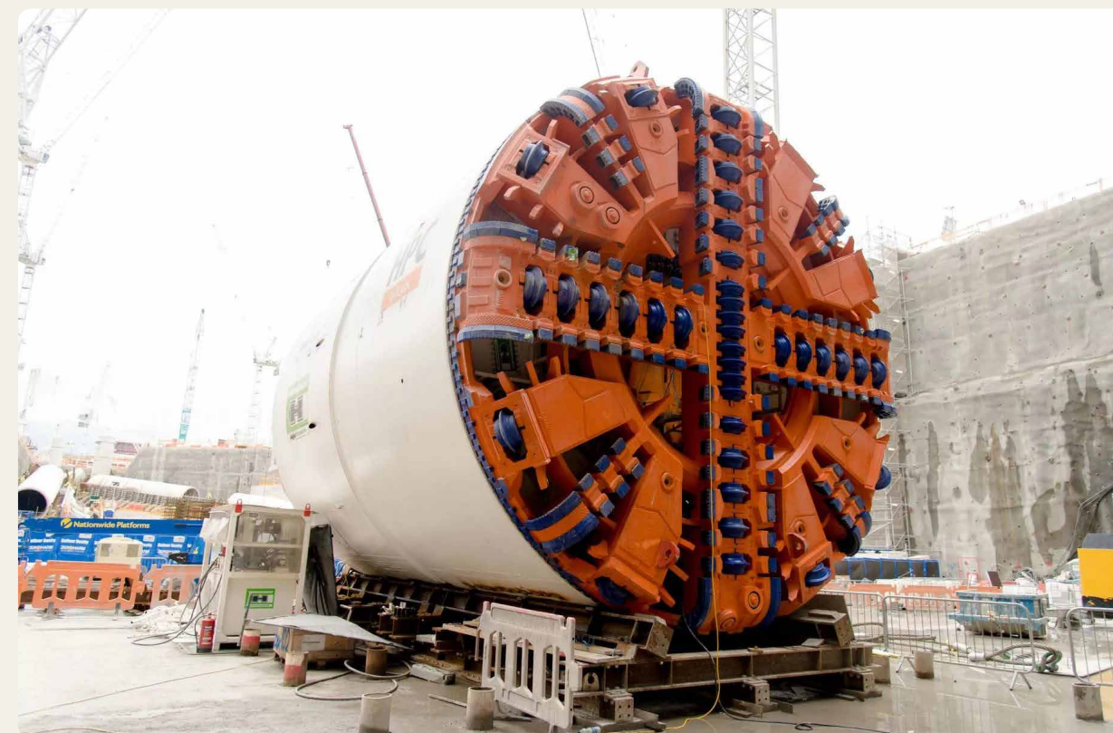
Figure 14. TBM used for HPC, giving an impression of dimensions. (Taylor, 2020)
